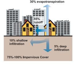
Relationship between impervious cover and surface runoff. Impervious cover in a watershed results in increased surface runnoff. As little as 10 percent impervious cover in a watershed can result in stream degradation.
